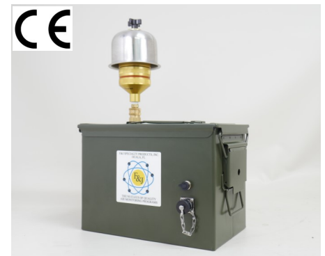
DF-ABM50-75L-20Li Military Grade AC/DC Air Sampler in Metal Ammo Box
