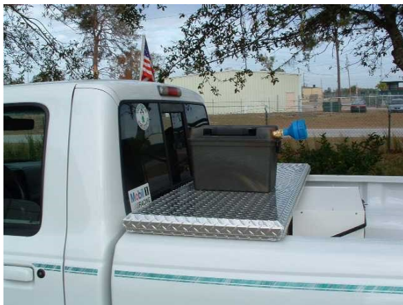
Connection to vehicle cigarette lighter for 12VDC sampling applications
