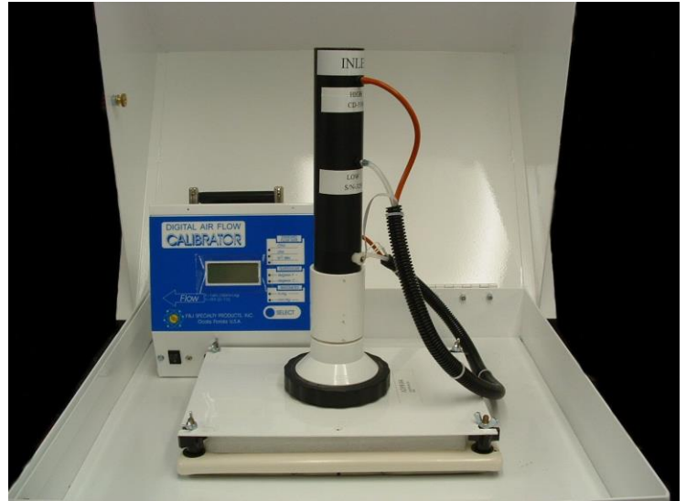
Calibration Setup for High Volume Air Sampler with 8"×10" Filter Holder
