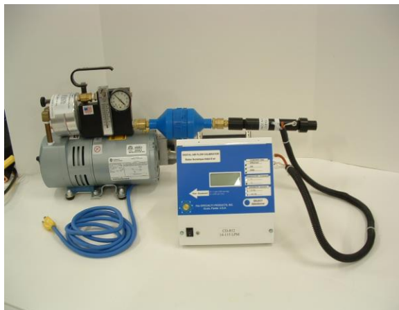
Calibration Setup for Portable Low Volume Air Sampler with Small Diameter Filter Holder
