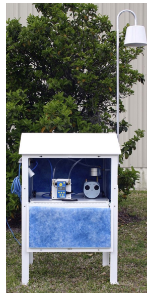
View inside weather house illustrating digital flowmeter
