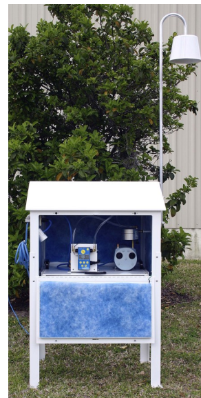
View inside weather house illustrating digital flowmeter
