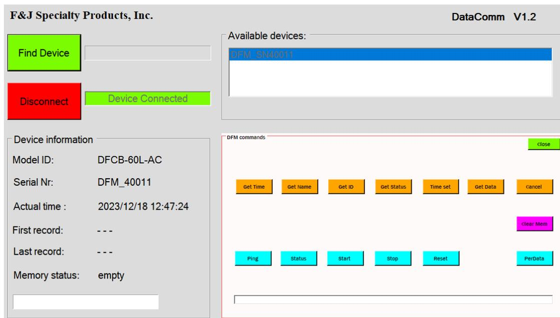
It is possible to send control commands and data requests to the DFM device by clicking on the orange or light blue buttons. The answer from the DFM can be viewed in the status line at the bottom of the white window. The available commands are listed below:
