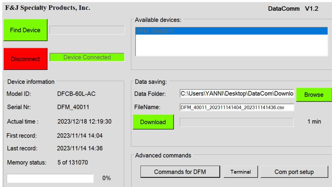
To start the data download, click on the "Download" button. The progress bar shows the actual status of the process, and next to the progress bar is the remaining time counter. The download process can be canceled at anytime, either on the computer or on the DFM. Although a download is cancelled, the partially downloaded data will be saved in the file location.
