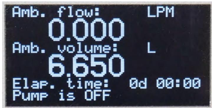
If the pump is running a "Pump is ON..." message will be displayed on the bottom of the menu. When the pump is running, the ambient flow rate ("amb. flow:") will display the current ambient flow rate of the air sampler in the factory set engineering units corrected to a set standard temperature and pressure (STP). The ambient volume will display the volume accumulated and will be changed accordingly as the pump is operating.
