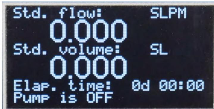
If the pump is running a “Pump is ON...” message will be displayed on the bottom of the menu. When the pump is running, the standard flow rate (“Std. flow:”) will display the current flow rate of the air sampler in the factory set engineering units corrected to a set standard temperature and pressure (STP). The standard volume will display the volume accumulated and will changed accordingly as the pump is operating.
