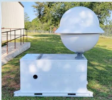
ULTRA High Volume CTBTO Air Sampler
