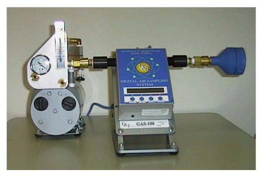
Model GAS-100-XX/100E-XX Series Units can be quick-disconnect-fitted to a conventional rotometer based unit.
