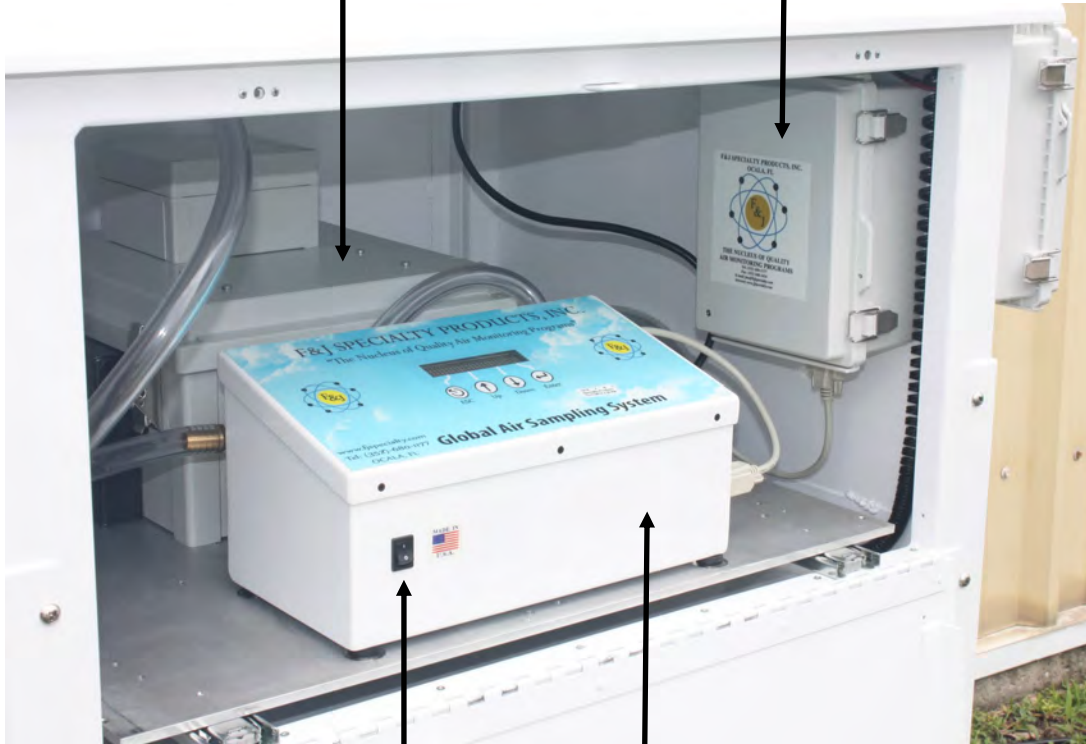
Global Air Sampler Flow Management System Electronic Module
