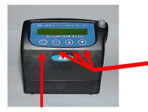
Press SET button and hold while using the Arrow keys to adjust flow
