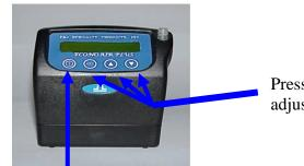
Press SET button and hold while using the Arrow keys to adjust flow
