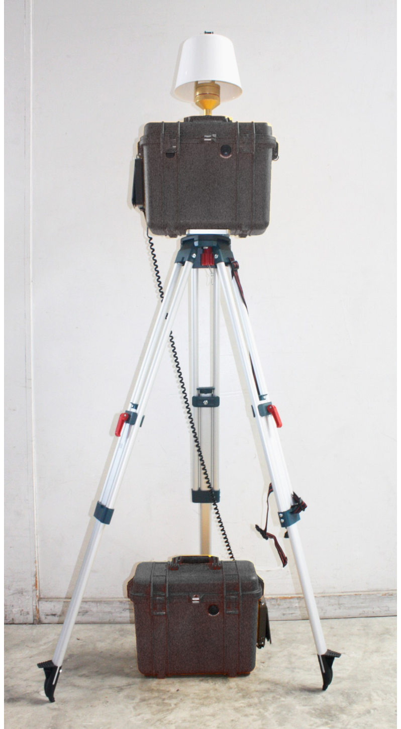
Air Sampler connected to LIBATBANK-12 portable battery bank
